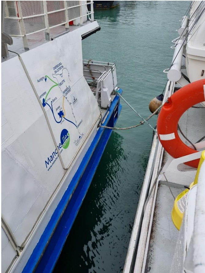
Arrangement of the vessels stern mooring at the time of the port state control inspection on 23 July 2023
