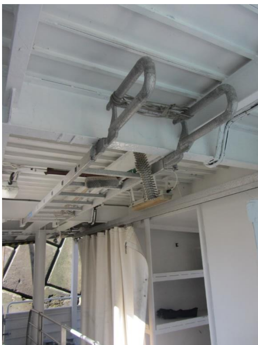
Vessels ladder used to access the shore when shore facilities are unable to be used.
